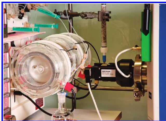
Figure 15. Setup for monitoring reactive intermediates during the Curtius rearrangement; the IR flow cell is attached between the first and second flow coil.
