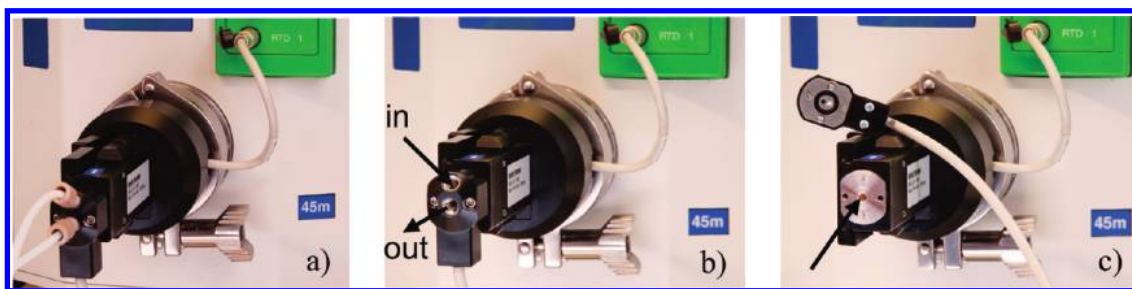
Figure 1. ReactIR 45m with prototype of IR flow cell attached. (a) Flow cell in line, connected with OmniFit adapters; (b) flow cell with OmniFit adapters removed, with direction of flow stream through the cell indicated; (c) head unscrewed, free view on diamond window (arrow).
